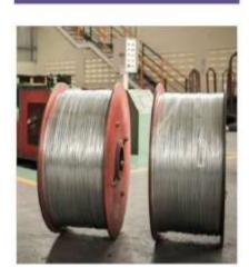
Kabatama Raya Armouring wires are produced by leveraging on the selected quality raw materials and the latest hot dipped technology to ensure the excellent and precision quality of galvanized wire for armouring cable purposes.
